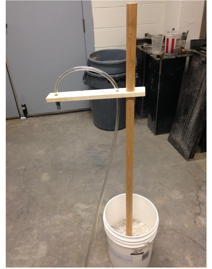
18. Thread tubing through the cross bar and jam the plastic plug into the end of the tube
