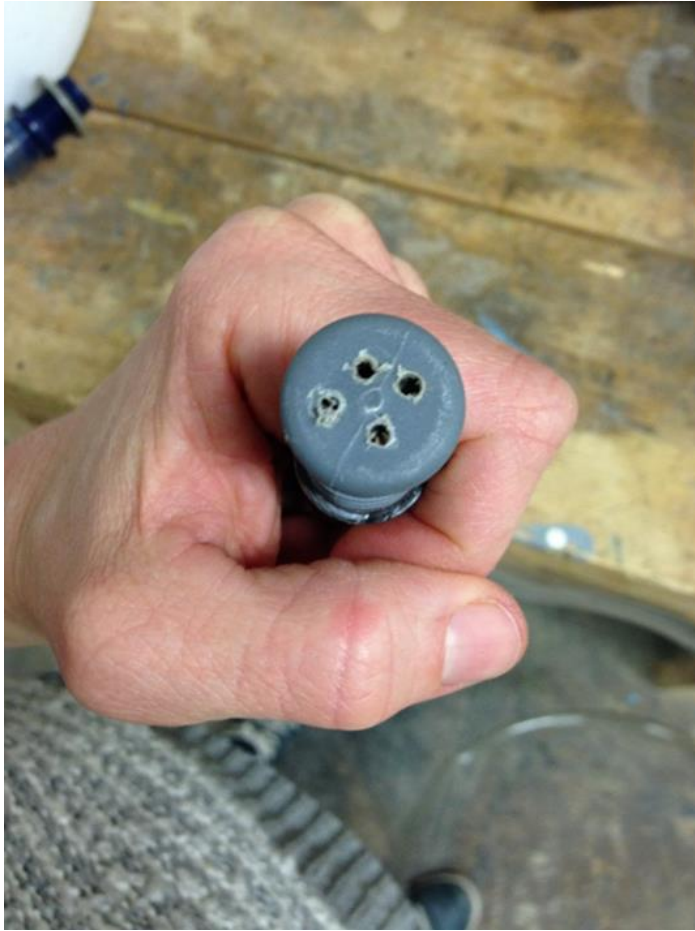
16. Drill several holes in the plastic plug
