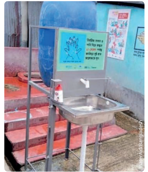
▲ Direct action pedal arrangement for soap and water dispenser.
