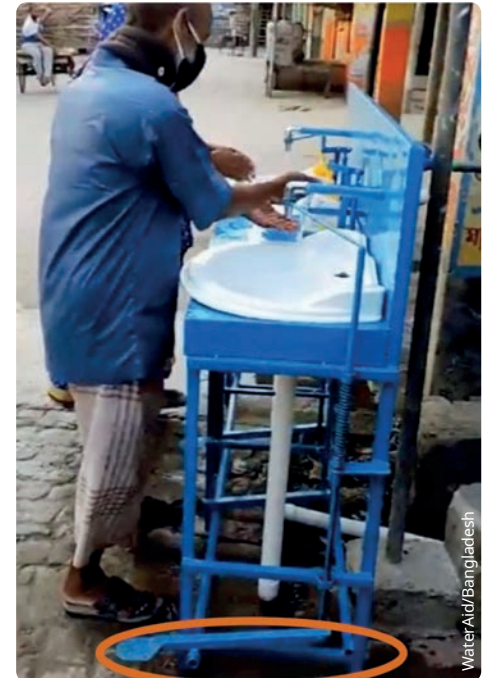
▲ A pedal arrangement working in an upward direction. Note the lift cock is getting a direct upward push in order to dispense water.
