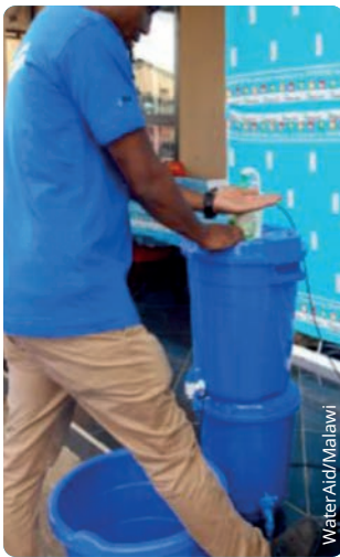
Figure 7: Pedal arrangement using bike brake cable to dispense water and soap (WaterAid Malawi).
