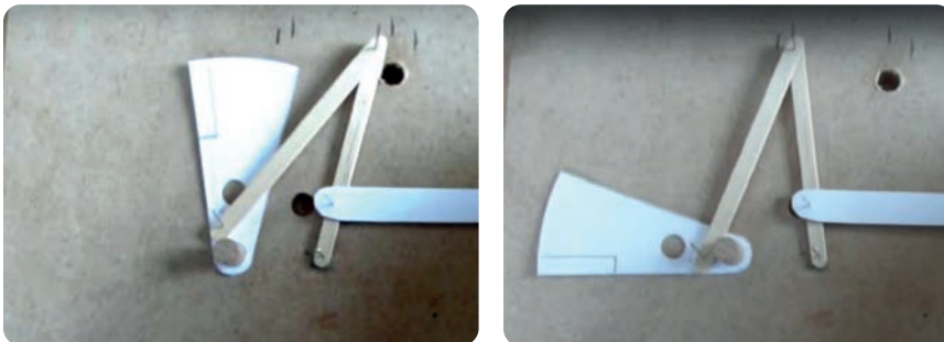
▲ Transition mechanism to translate linear movement to rotation (see this video for more details: youtube.com/watch?v=09jZsBDHaIE ).
